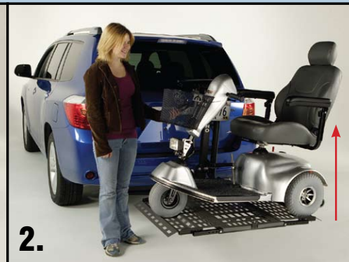
Raise lift to automatically secure scooter.
